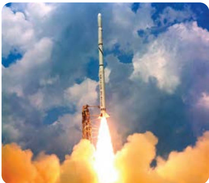
Four-stage, solid propellant Scout rocket.
