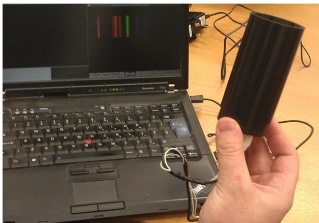
Figure 20.1: This is one type of digital spectroscope that you may be using. Be sure to avoid touching the lens portion of the instrument.
